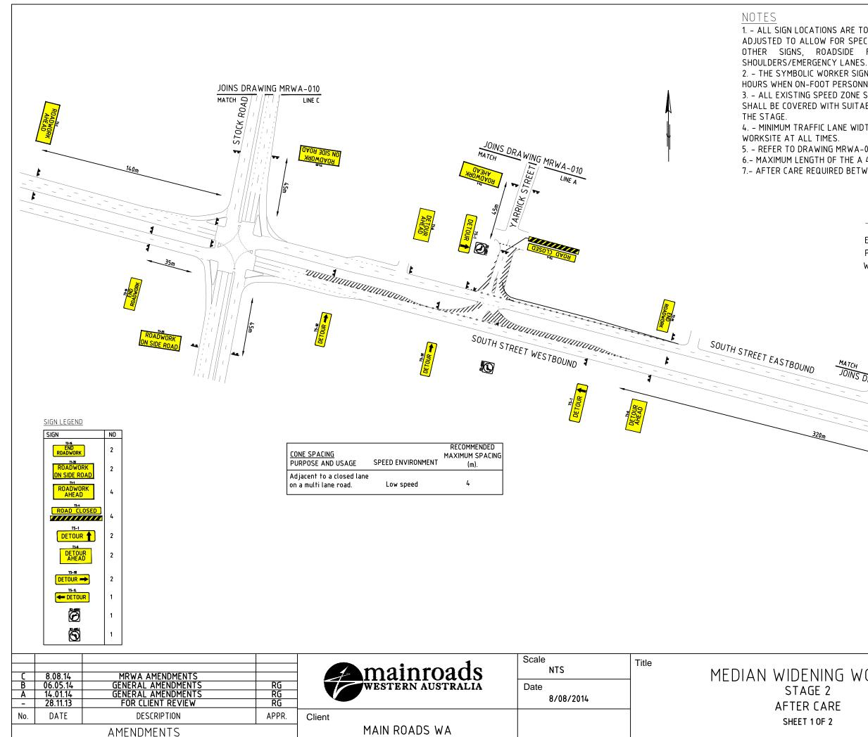
1. - ALL SIGN LOCATIONS ARE TO BE CHECKED PRIOR TO SETOUT AND POSITIONS ADJUSTED TO ALLOW FOR SPECIFIC SITE CONSTRAINTS SUCH AS VEGETATION, OTHER SIGNS, ROADSIDE FURNITURE AND SUFFICIENT SPACE ON SHOULDERS/EMERGENCY LANES.
