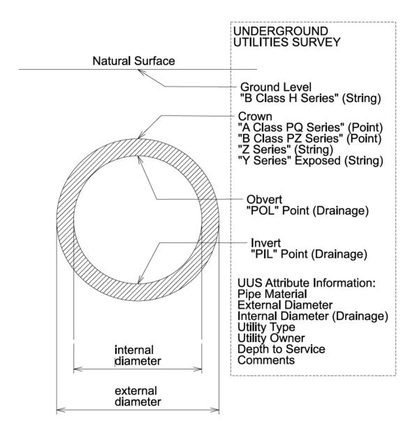
A bank of services that follow one alignment should be described on the Utility Plot and text added to the GenIO. A diagram showing the bank should be placed at start and end pits on the Utility Plot, which describes the layout (e.g., 4x2 P40), the utilities contained and which service was traced / located. Photos of the bank are also acceptable provided they clearly show the services and are annotated.
