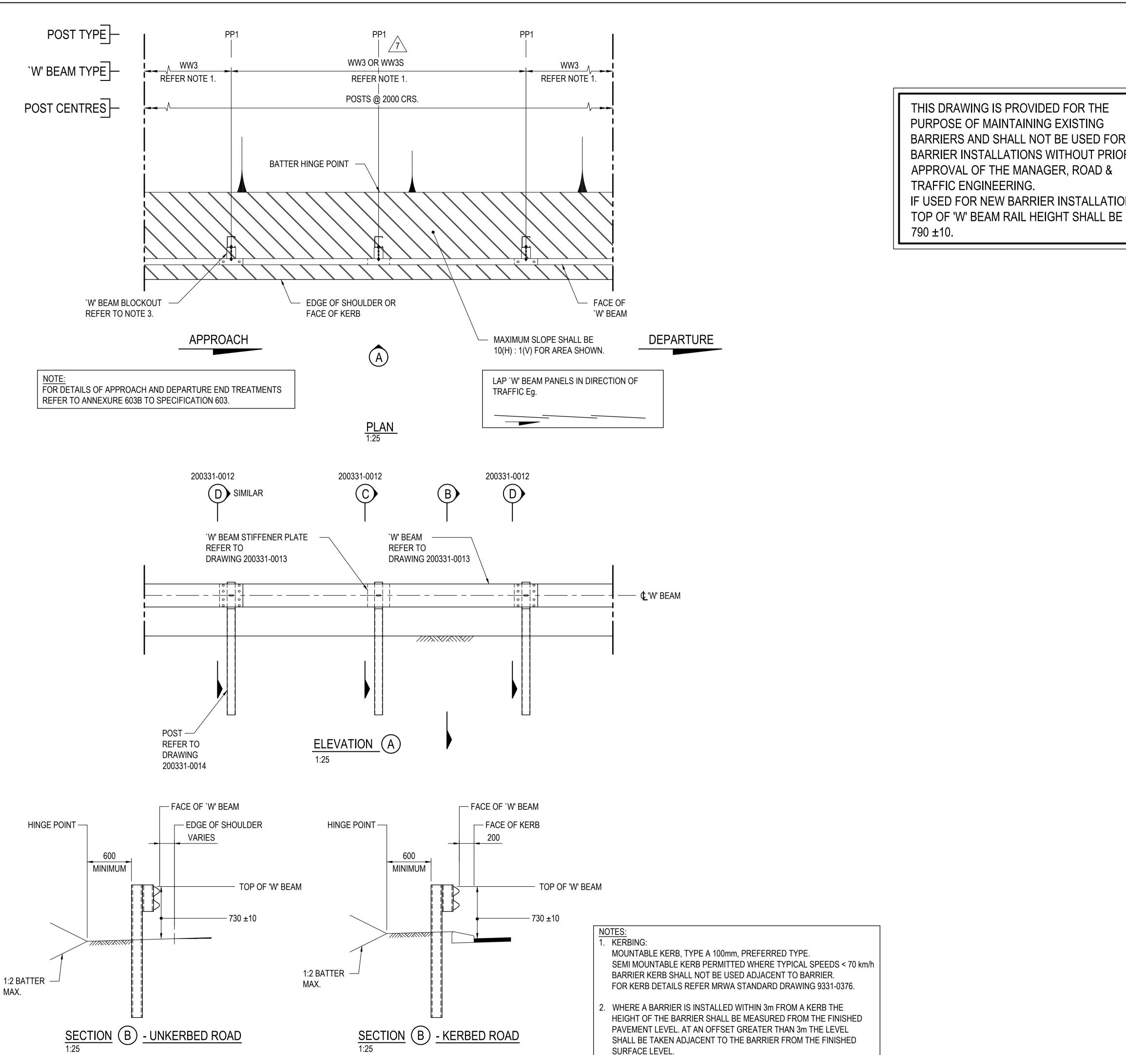
THIS DRAWING IS PROVIDED FOR THE PURPOSE OF MAINTAINING EXISTING BARRIERS AND SHALL NOT BE USED FOR NEW BARRIER INSTALLATIONS WITHOUT PRIOR APPROVAL OF THE MANAGER, ROAD & TRAFFIC ENGINEERING. IF USED FOR NEW BARRIER INSTALLATIONS,
