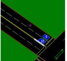
Detector 9 (shared through/left turn lane) – 400 veh Detector 10 (shared through/right turn lane) – 350 veh Total detected – 750 veh Using the turning proportions from the survey count: Left turn – 27% = 204 veh Through – 57% = 430 veh Right turn – 15% = 116 veh
