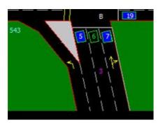
Detector 5 (through lane) – 500 veh Detector 6 (through lane) – 450 veh Detector 7 (shared through/right turn lane) – 150 veh Total detected – 1100 veh
