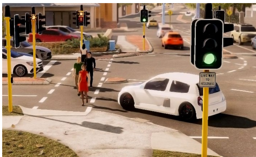
Image 4: Conflicting, turning vehicles giving way to pedestrians after the LPI period with FYCL in operation
