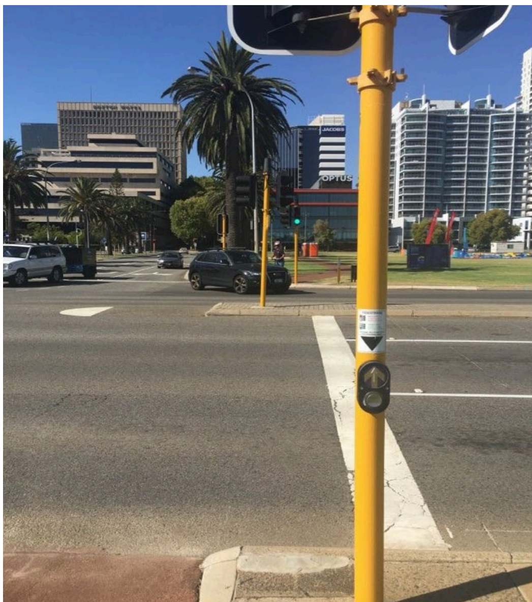
Figure 8: An example pedestrian crossing with no pedestrian aspects, with a traffic roundel display for pedestrians
