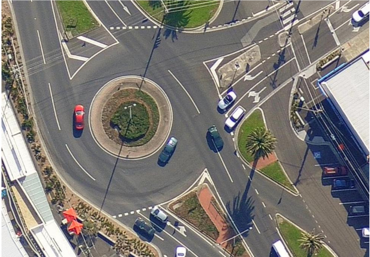
Figure 6.3: Roundabout Metering Using Pedestrian Operated Signals on Approach Leg only and Zebra Crossing on Exiting Leg
