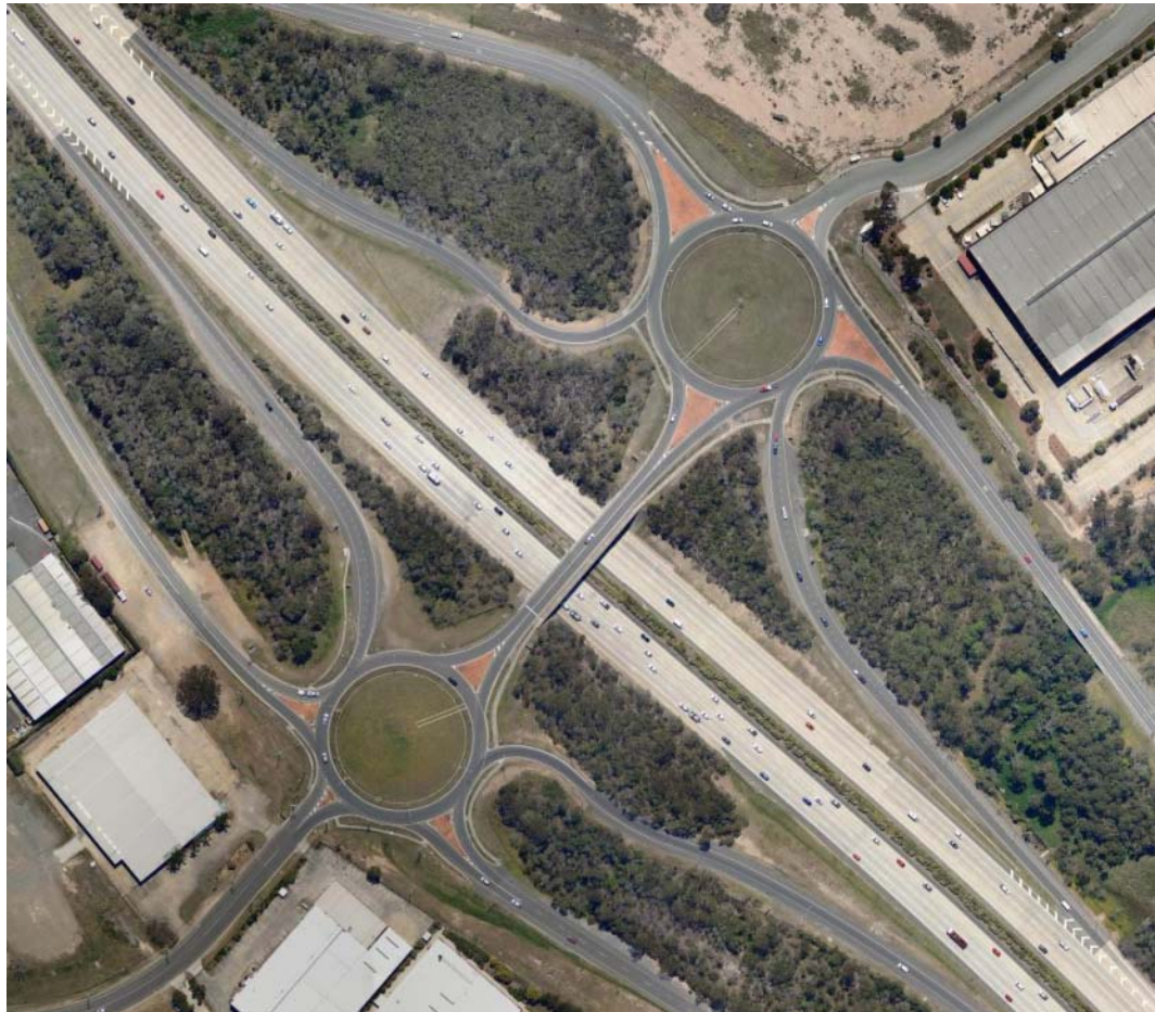
Figure A.2: Example of Two Single-lane Roundabouts with Six Legs Each Ormeau, Qld
