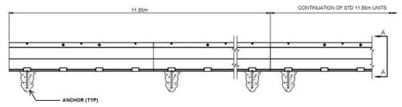
Plan and Elevation of Anchored ZoneGuard MDS End Unit
