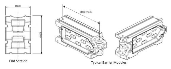
Figure 2: Typical Details of Shield I Barrier
