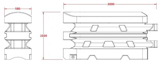
Figure 2: Typical Details of Ricochet Barrier
