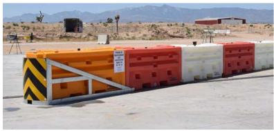
Figure 1: Photograph of Lo-Ro Barrier and SLED Lo-Ro Terminal
