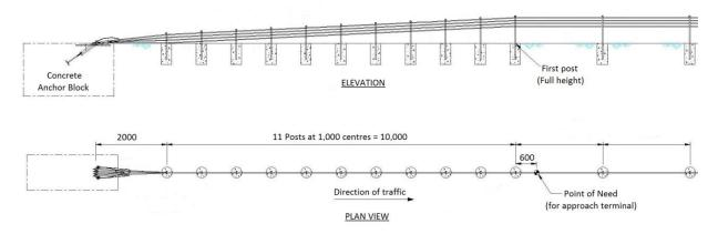
Flexfence TL3 Terminal (refer to Supplier for Concrete Anchor Block details)
