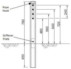
Flexfence TL4 4 Wire Rope Barrier - Typical Cross Section
