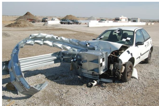
Crash test photograph showing w-beam extruded onto traffic side.
