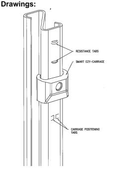
Isometric View – Z Posts and Ezy-Carriage (W-beam omitted for clarity)
