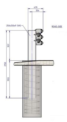
**Typical Cross Section thru Abutment Post**
