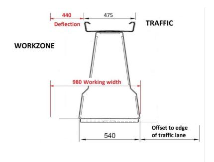
Deflection and Working Width shown in Cross Section
