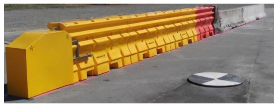
Photograph of Armorbuffa System (4 Water Filled Elements)
