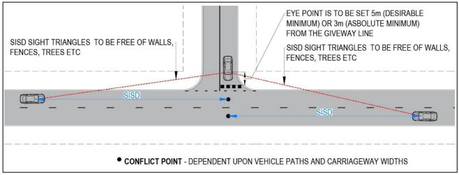
Figure 3.2 (Plan Only): Safe Intersection Sight Distance (SISD)
