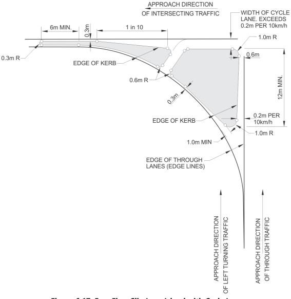
Figure 6.17: Free Flow Slip Lane Island with Cycle Lane
