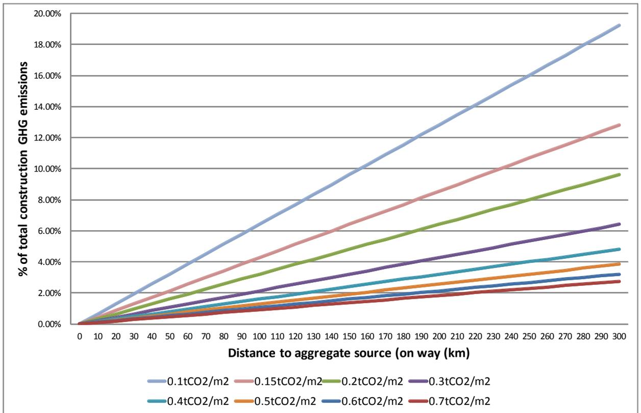
**Figure 3.7 Transport of aggregate percent contribution to construction GHG emissions**
