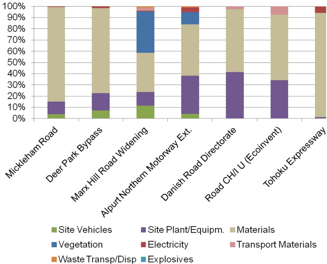
**Figure 3.6 Road construction – breakdown of emissions**
