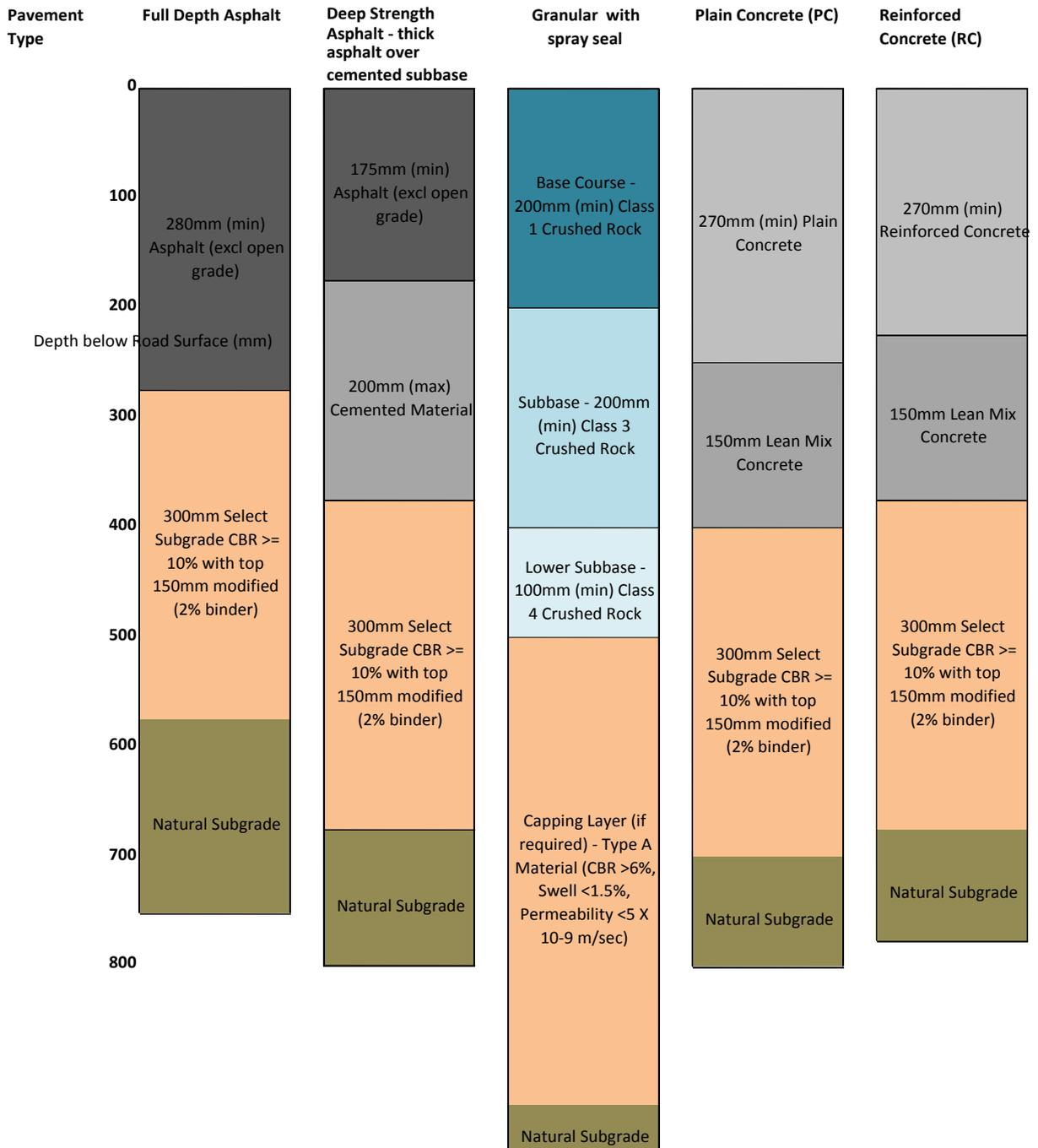
Figure 4.3 Pavement types and material depths
