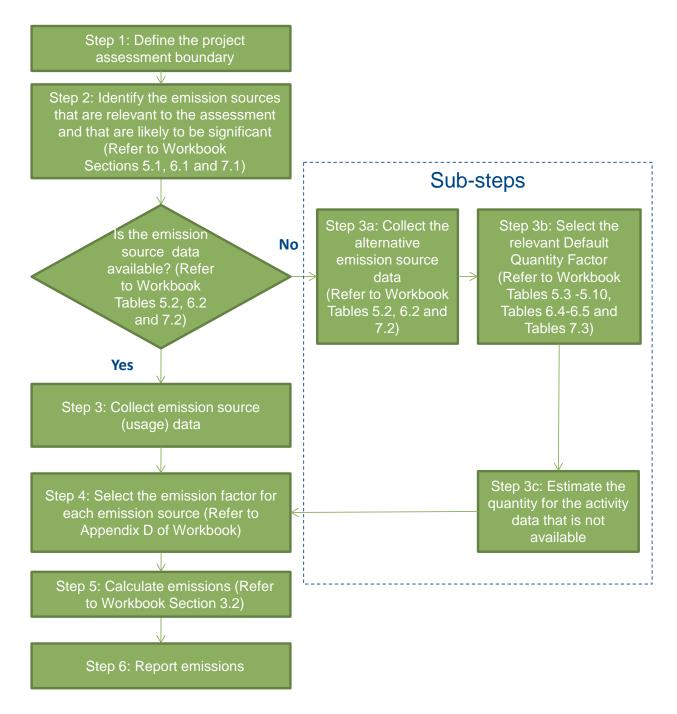
Figure 2.1 Overview process for calculating GHG emissions
