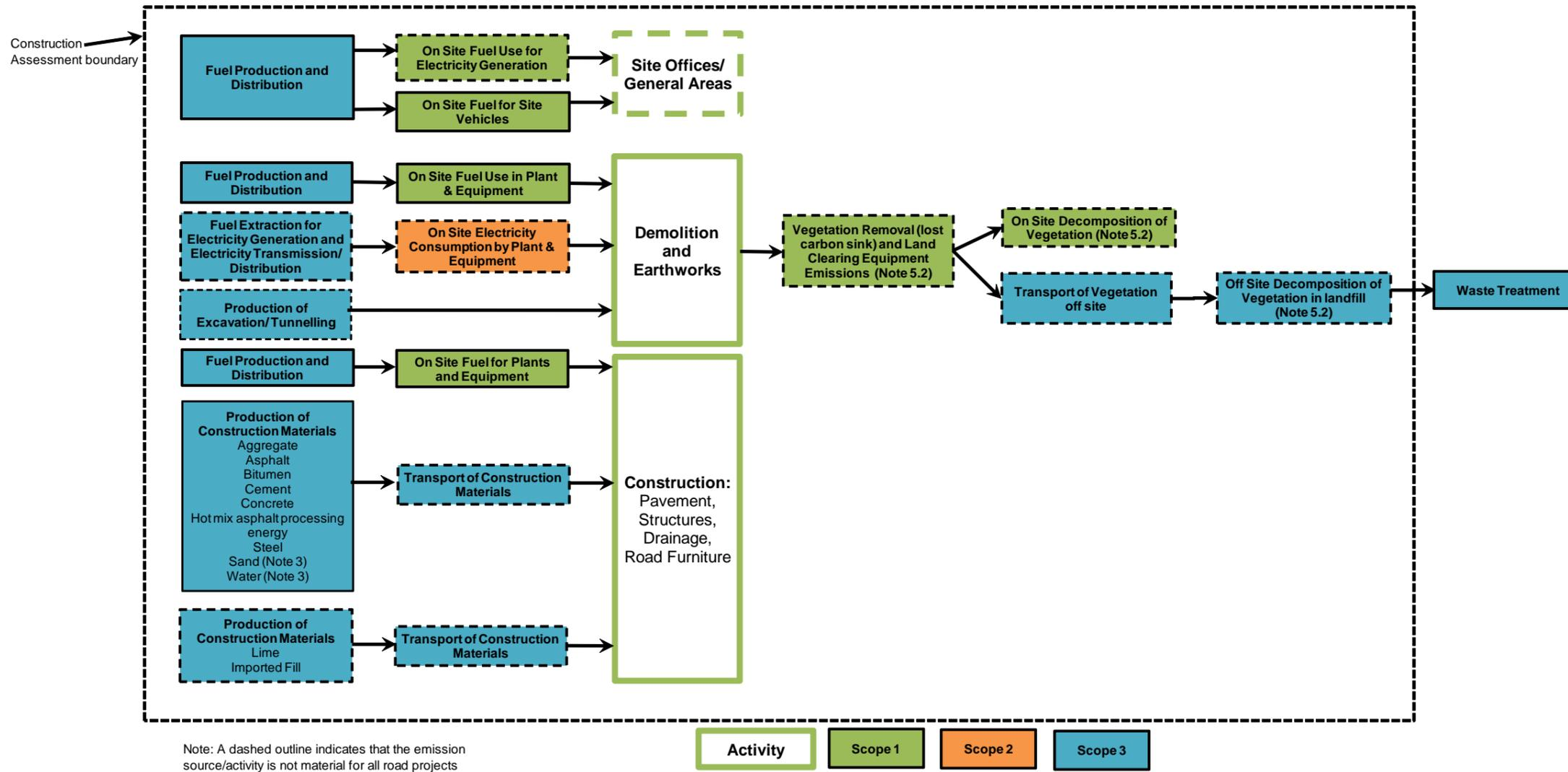
Figure 5.1 Construction GHG assessment boundary
