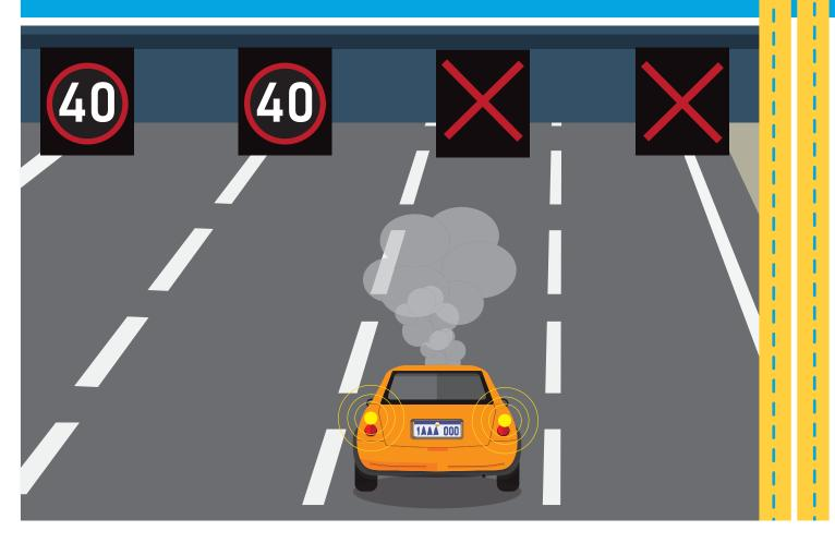
There are 12 overhead electronic sign structures on our new Smart Freeway, between the Mt Henry Bridge and the Narrows Bridge. These are designed to keep motorists informed, adjust speed limits and close lanes when needed, to help traffic flow more smoothly.
