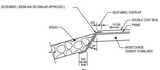
DETAIL ① GEOFABRIC DETAIL AT ROCK PROTECTION FLOODWAY TYPE 2
