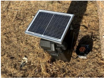
Above: Vibration monitor set up on site.
