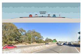
In locations where there are constraints on both sides, such as development or environmental issues, a narrow median with concrete barrier would minimise impacts.
