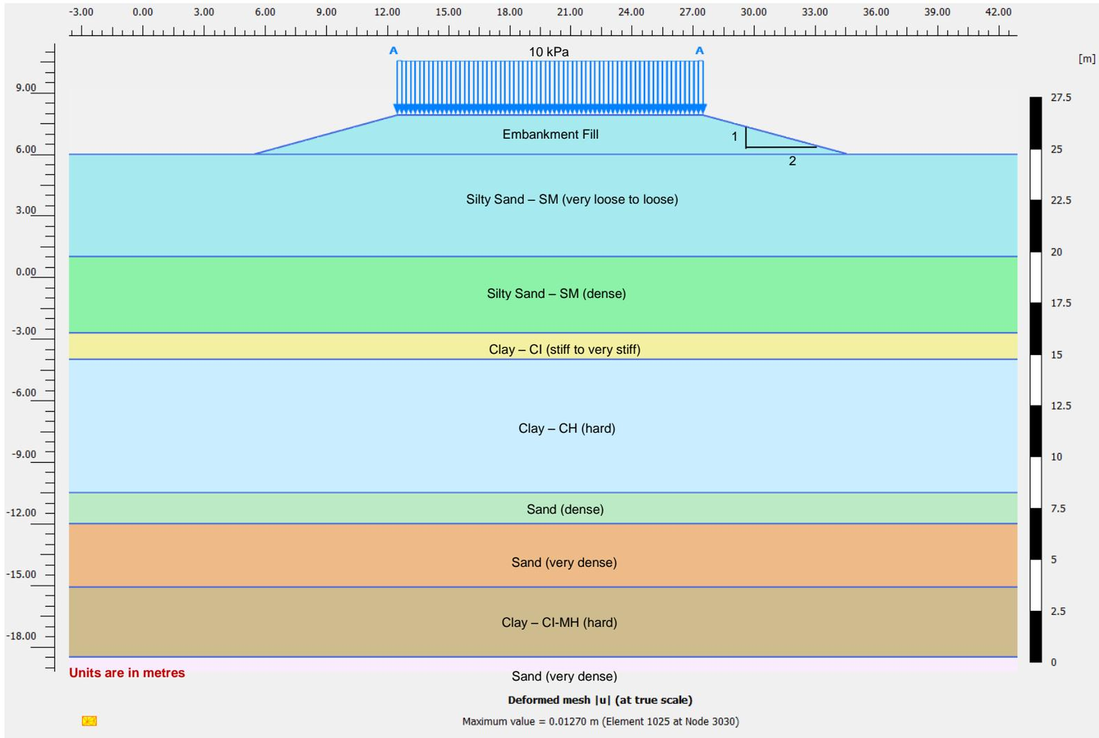
Plate 1 Soil Model for Eastern Approach Embankment of Bridge 1763
