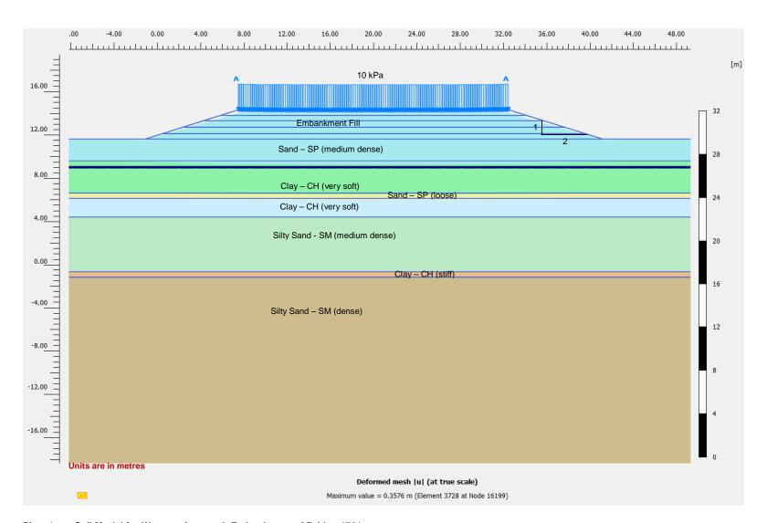
Plate 1 Soil Model for Western Approach Embankment of Bridge 1761
