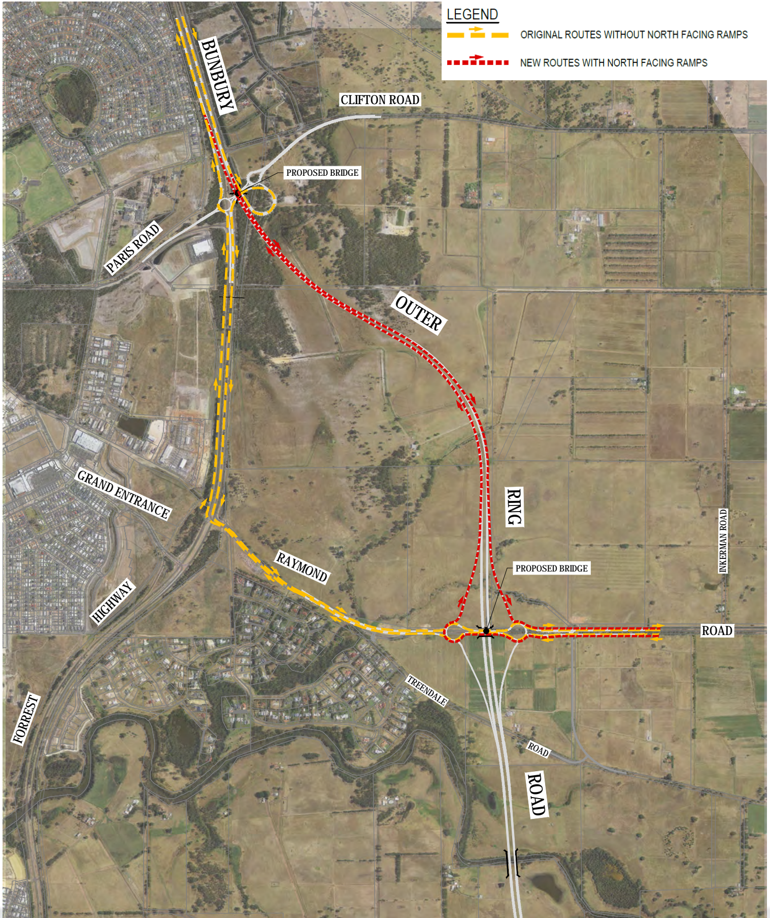
Figure 2 Route comparison with and without northern ramps at Raymond Road interchange with BORR.
