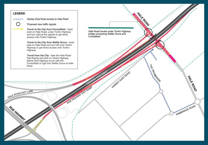
This new design concept uses a lower speed limit on the side road to provide direct access to Tonkin Highway northbound from Hale Road without compromising safety.
