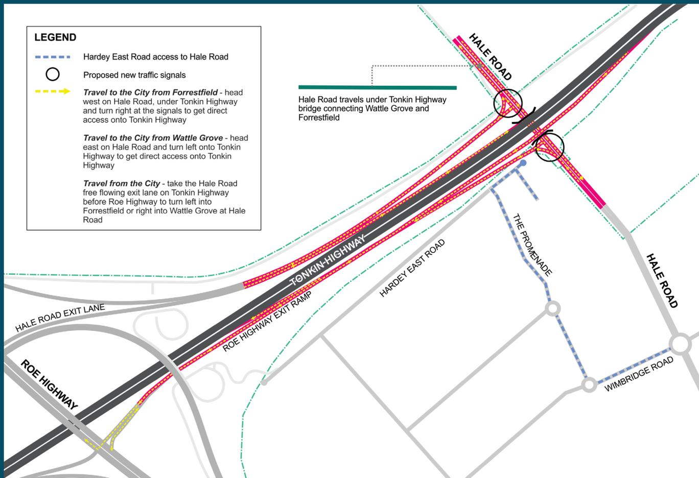
**This new design concept uses a lower speed limit on the side road to provide direct access to Tonkin Highway northbound from Hale Road without compromising safety.**
