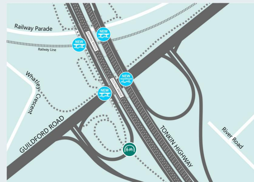
There are 60 bridge beams to be installed for the four new bridges over Railway Parade and Guildford Road - the biggest being 35 metres long and weighing 135 tonnes.
