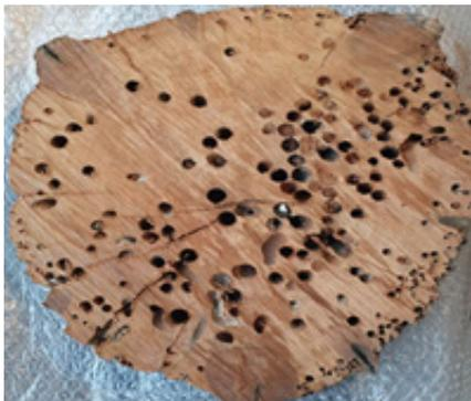
Teredo worm activity on exposed timber below failed concrete encapsulation
