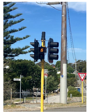
Figure 1: Pedestrian Countdown Timers at Marmion Street and Stirling Highway.
