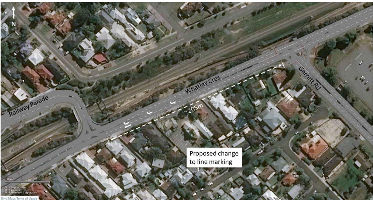
Figure 2-8 Whatley Crescent / Railway Parade Proposed Line Marking
