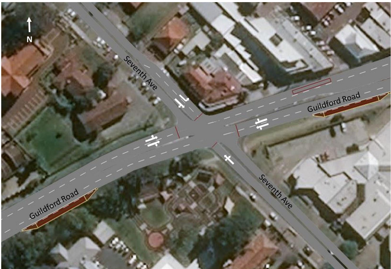
Figure 2-4 Guildford Road / Seventh Avenue Proposed Intersection Layout
