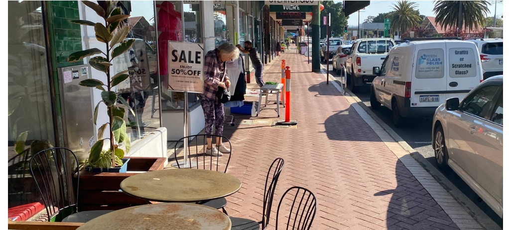
Footpath width squeezed by overly large road pavement
