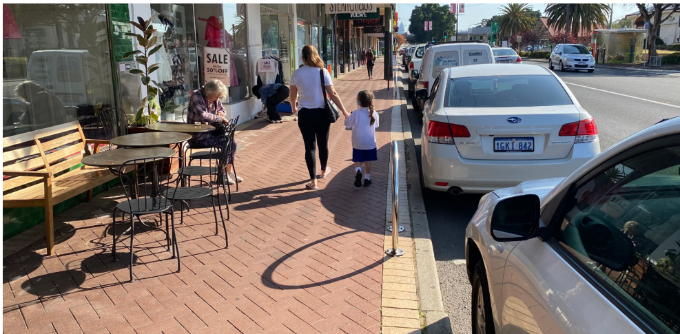
High traffic areas require a wider footpath so two people can walk side by side and a wheelchair or mobility scooter can pass in the opposite direction
