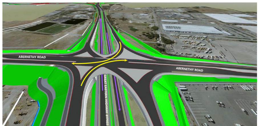
The second movement involves opposing left-turn lanes from the bypass and/or exit travelling through the traffic signal on to Abernethy Road.
