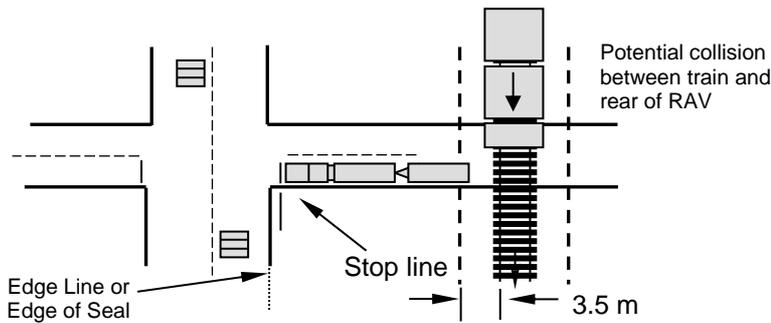
Figure 4: Examples of Inadequate Departure Stacking Distance
