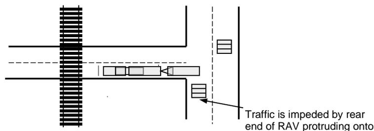
**Figure 3: Examples of Inadequate Approach Stacking Distance**
