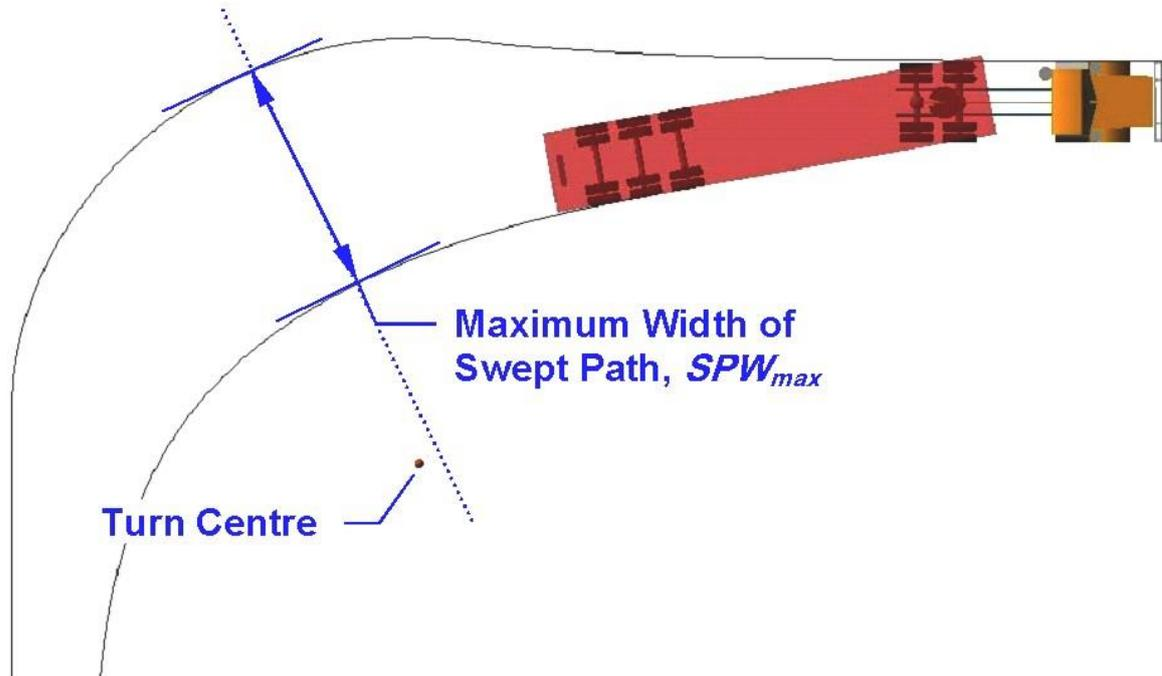
**Figure 6.** Plan view illustration of Maximum Width of Swept Path,  $SPW_{max}$ . Note that the line perpendicular to both path trajectories (shown dotted in the illustration) does not necessarily pass through the turn centre.
