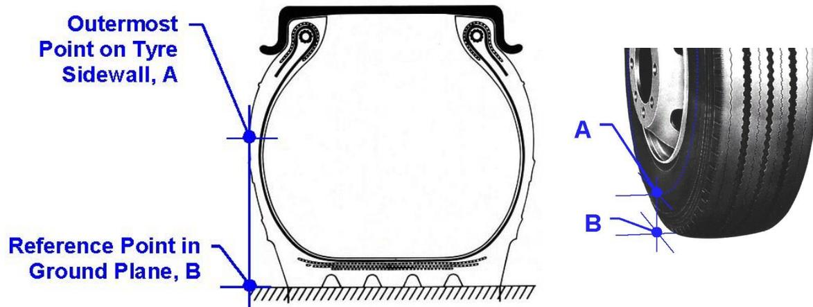
Figure 7. Illustration of outside wheel reference point.
