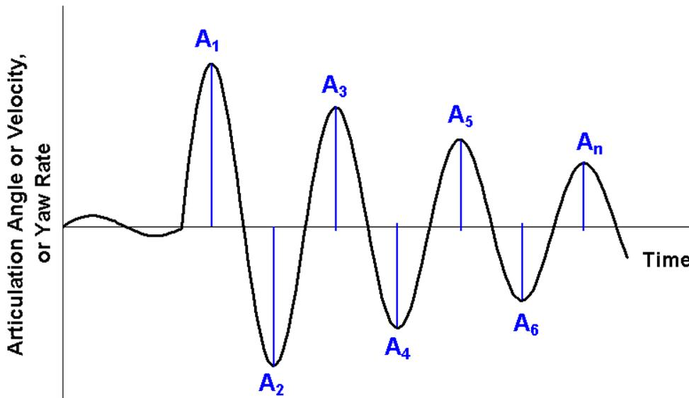
Figure 20. Determination of amplitudes for damping ratio calculation.
