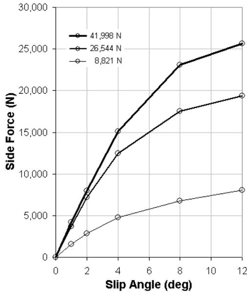
**Figure 22. Side force characteristics of an 11R22.5 size truck tyre showing the influence of tyre vertical load.**
