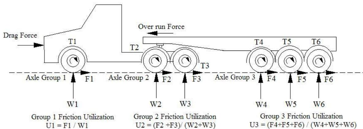
The brakes generate retardation torques T1...T6.
