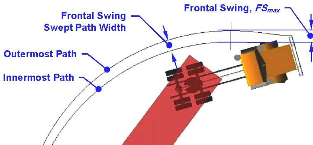
**Figure 8.** Illustration of path trajectories in the Performance Based Standards low-speed turn of Part A of the frontal swing performance measure. For this measure the innermost path is the path followed by the outside front wheel.
