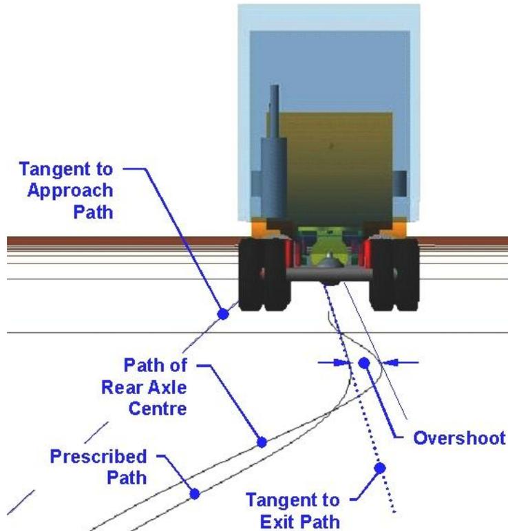
**Figure 18.** Perspective view illustration of final stages of the single lane change manoeuvre showing overshoot dimension in the ground plane of the rear axle centre for high-speed transient offtracking.
