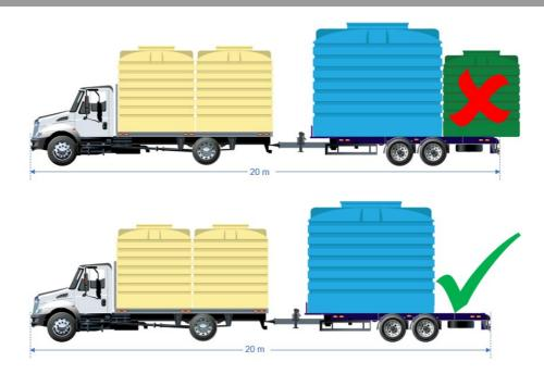
**2.2.6** Multiple items must not be loaded front to back on a rigid truck and dog trailer combination, if it results in the length exceeding 25 metres in overall length or an allowable vehicle dimension limit, such 12.5 metres for the rigid vehicle, or 3.7 metres rear overhang.
