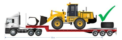
**2.2.5** Multiple items must not be loaded front to back on a rigid truck and pig trailer (or tag trailer) combination if it results in the length, measured from the front of the vehicle combination to the rear of the load, exceeding 20 metres in overall length or an allowable vehicle dimension limit, such 12.5 metres for the rigid vehicle, or 3.7 metres rear overhang.
