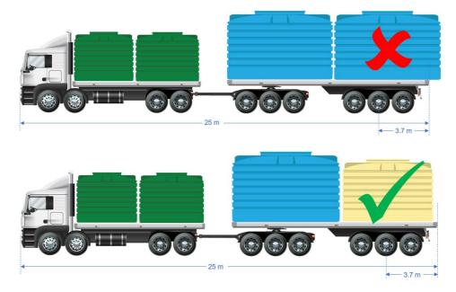
**2.2.7** Multiple items must not be loaded front to back on a road train or B-double, if it results in the length exceeding the allowable road train or B-double overall length or an allowable trailer dimension, such as 3.7 metres rear overhang.
