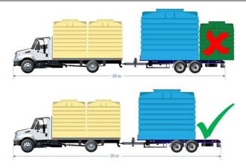
**2.2.6** Multiple items must not be loaded front to back on a rigid truck and dog trailer combination, if it results in the length exceeding 25 metres in overall length or an allowable vehicle dimension limit, such 12.5 metres for the rigid vehicle, or 3.7 metres rear overhang.
