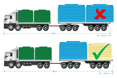
2.2.7 Multiple items must not be loaded front to back on a road train or B-double, if it results in the length exceeding the allowable road train or B-double overall length or an allowable trailer dimension, such as 3.7 metres rear overhang.
