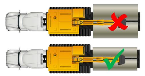
**2.1.2** Multiple items must not be loaded side by side if it results in the overall width exceeding 2.5 metres, regardless of the trailer width.
