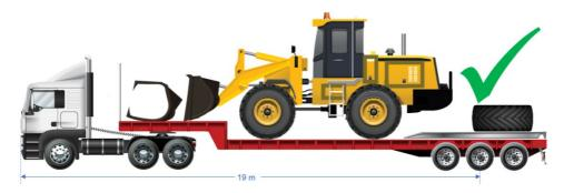
2.2.5 Multiple items must not be loaded front to back on a rigid truck and pig trailer (or tag trailer) combination if it results in the length, measured from the front of the vehicle combination to the rear of the load, exceeding 20 metres in overall length or an allowable vehicle dimension limit, such 12.5 metres for the rigid vehicle, or 3.7 metres rear overhang.
