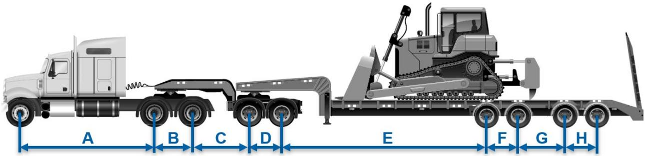
**6.2.2** If the vehicle combination consists of a twin steer prime mover, the axle spacing “A” measurement must be taken as per the following diagram.
