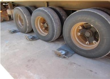
It is important to remember that weighing must take place on firm, level ground and suspension torque must be managed to ensure the weights determined are correct each time.
