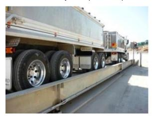
Some weighbridges have multiple decks allowing the vehicle's axle groups to be weighed simultaneously and software systems that provide the driver with printed dockets showing these weights.
