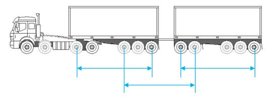
"Single Axle" does not include a single steer axle. "Tandem axle group" does not include a twin steer axle group.
