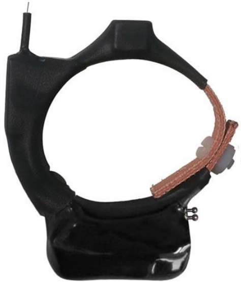
Figure 10. Lotek LiteTrack 30 collar
