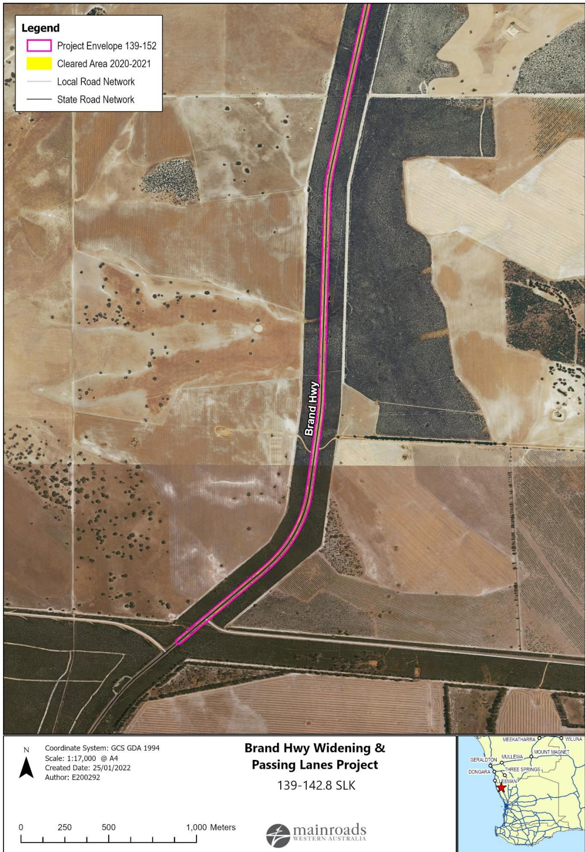
Figure 4: Clearing completed between 139-142.8 SLK (Plan 7533/2n)
