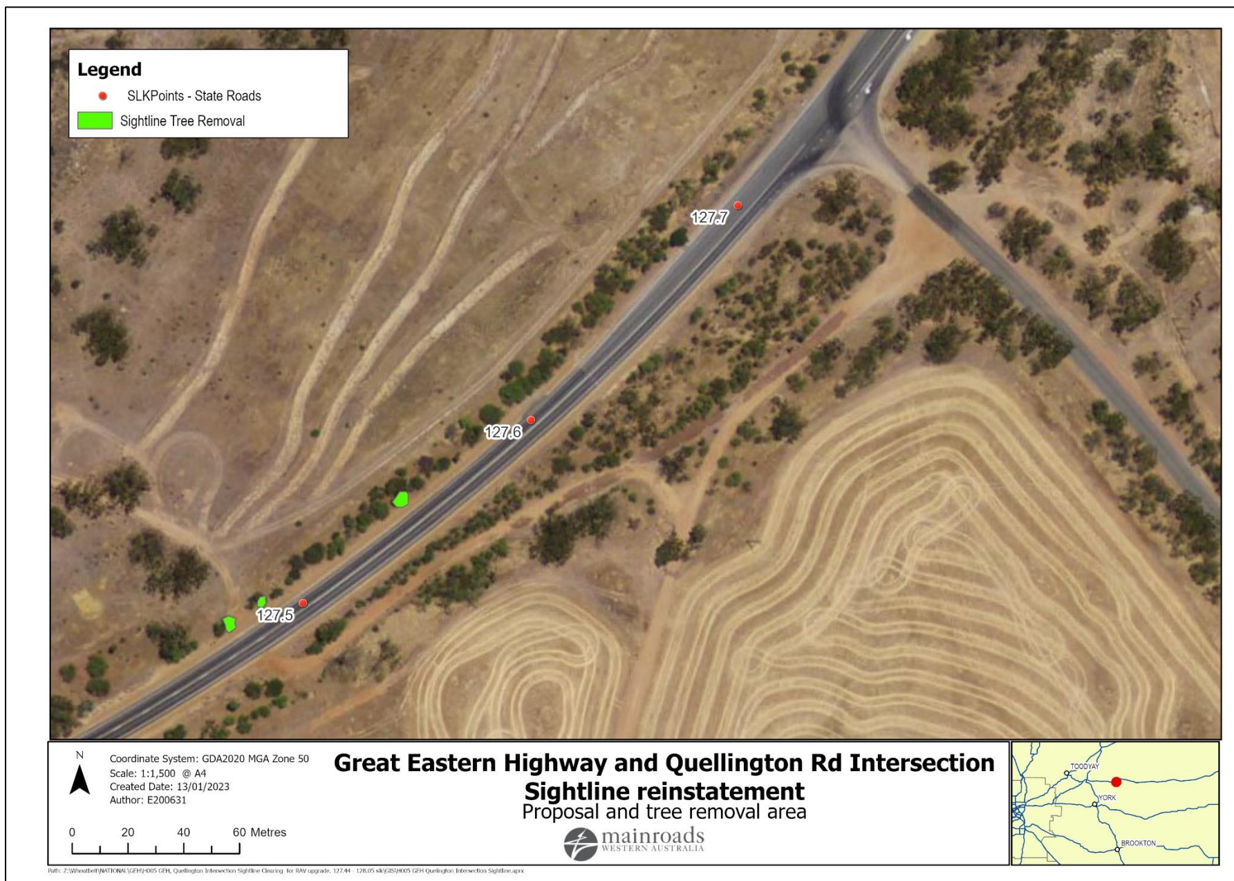
Figure 1: GEH and Quellington Rd Intersection Sightline reinstatement (127.44-127.80 SLK)
