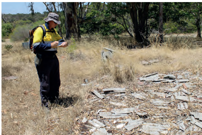
IMG_0090 .....400356 mE 6484121 mN Concrete slab, toilet block with asbestos roofing (very fragmented); Asbestos fencing as well with D. Cooper.
