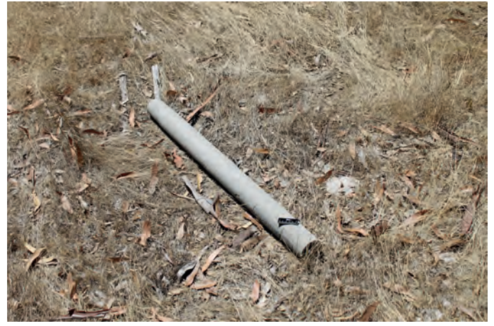
IMG_0121 .....400391 mE 6484254 mN Asbestos-lined pipe.
