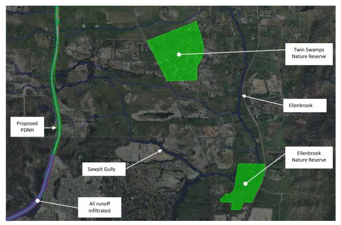
Figure 4: Surface flow patterns from PDNH
