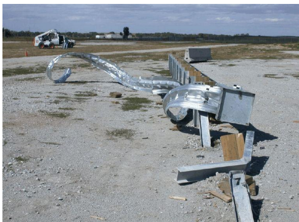
Crash test photograph showing w-beam extruded onto verge side
