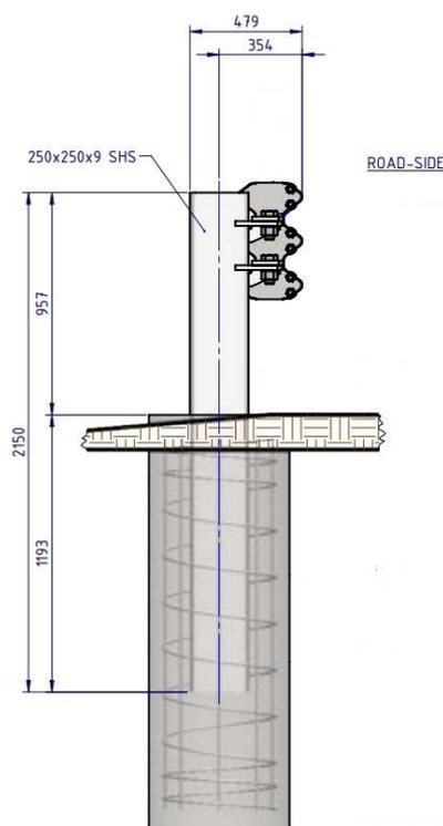
Typical Cross Section thru Abutment Post
